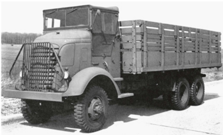
Factory photo of a GMC AFKW-353 COE truck with 17-ft. platform body (M427), taken in 1944. The U.S. Army registration number 4289577 is of special interest as it does not fit into the range of serial numbers assigned to the 4,000 vehicle contract of the late model AFKW-353 but was instead assigned to a CCKW-352 cargo truck w/ winch. The platform body is a metal-reinforced wood structure with removable front and side racks. Folding troop seats, incorporated in the side racks, permit the transport of both personnel and general cargo. Seven top bows are used on the 17-ft. platform body. (GMC Truck and Coach Division)
