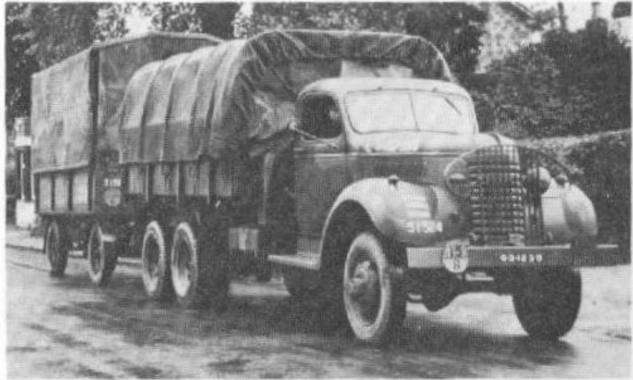
Truck, 3-ton, 6×6, Cargo (GMC ACKWX-353) 6-cyl., 77 bhp (net), 4F1R×2, wb 175 \frac{3}{4} (BC 44) in, 264×94 \frac{1}{2} ×118(90) in, 9856 lb. Another 'ex-French' type, diverted to Britain in 1940. US Army had similar trucks with 162-in wb and US standard type cargo body. IWM photo H24419.
