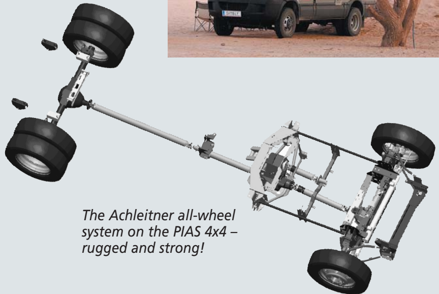
The specially developed Achleitner front axle beam
