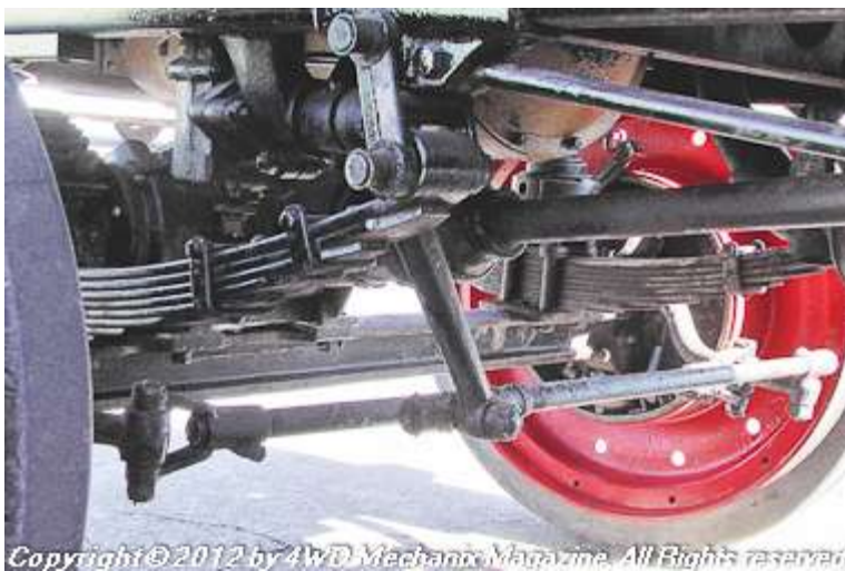
The manual steering gearbox has a worm and sector to move the pitman arm. Leaf springs have shackles like Jeep leaf spring suspension.
